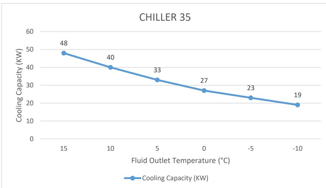
This 'de-rate table' is a rough guide as to chiller cooling capacity at different outlet fluid temperatures allowing for quick selection on applications. It is based on a 30°C ambient temperature and glycol mix to suit outlet temperature. For accurate selection we are able to run a full selection on your application.
