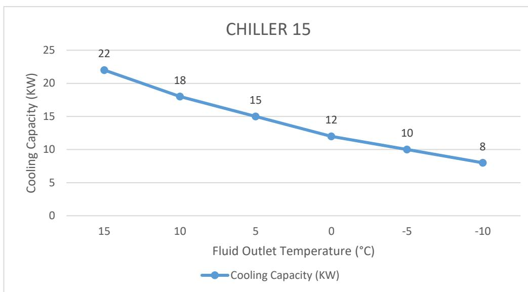
This 'de-rate table' is a rough guide as to chiller cooling capacity at different outlet fluid temperatures allowing for quick selection on applications. It is based on a 30°C ambient temperature and glycol mix to suit outlet temperature. For accurate selection we are able to run a full selection on your application.
