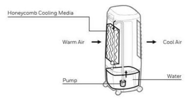
The recommended maximum relative humidity level is 60% or less, which allows a noticeable temperature decrease. The temperature will be lower in drier climates because higher evaporation occurs when the humidity is low.
